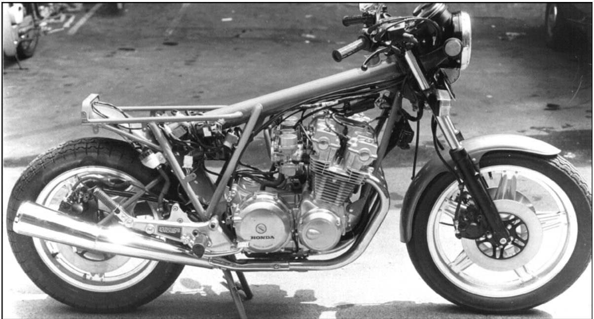
This Foale frame used a large backbone above the engine, with triangulated support for the swing-arm pivot.
