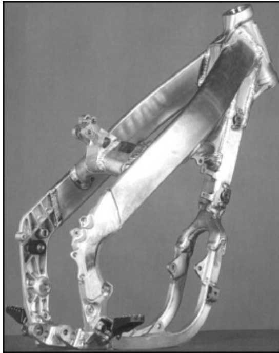
Above: The 1998 Kawasaki Ninja used a twin-spar frame very little different from its main competitors shown above. Note that in common with the R1 and Hayabusa the front engine mounting is quite high up, rendering traditional down-tubes and bottom cradle unnecessary, thereby freeing up valuable space.
