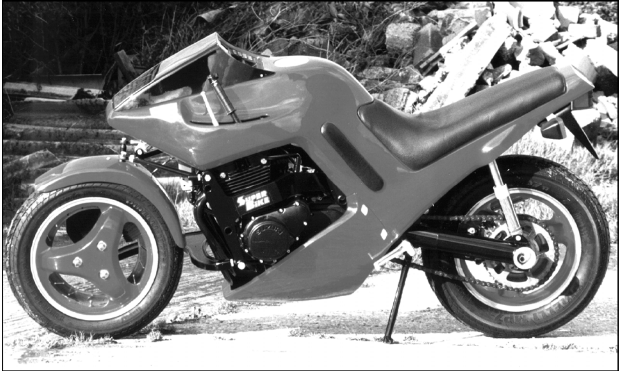
Showing the above single sided arm fitted to the Q2. Suspension was by means of a single Fournales air shock attached close to the rear of the arm.
