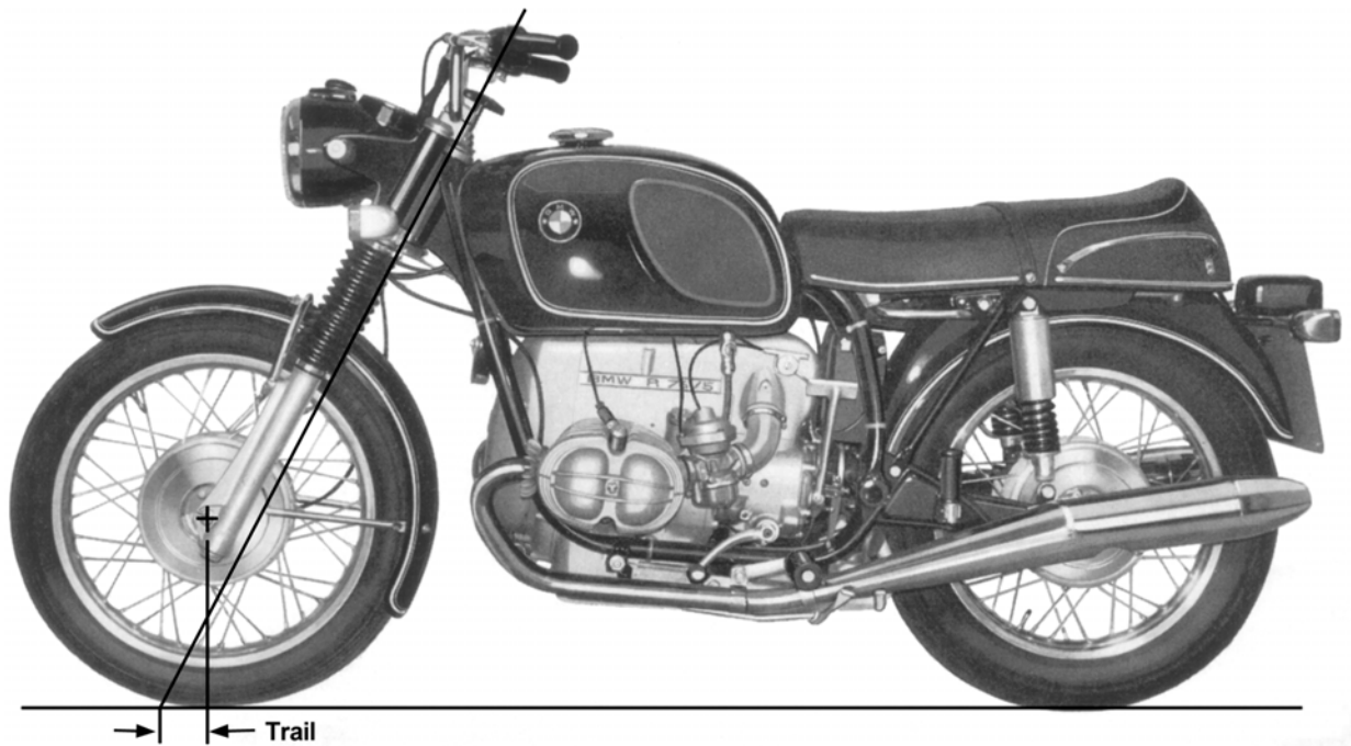
The standard BMW R75/5 used as a basis for the experiments in rake and trail, maker's figures were 27 degrees rake and 89 mm. ground trail.
