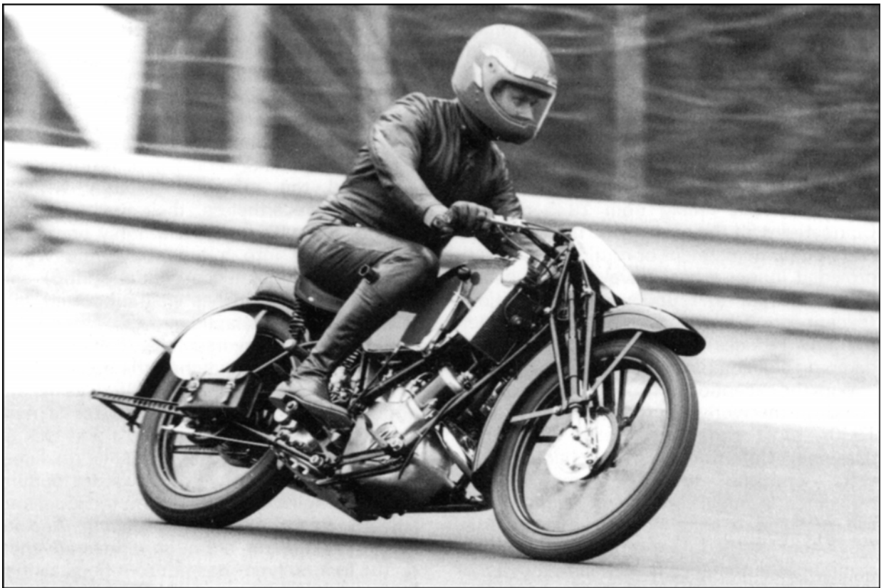
Manfred Schweiger's 1929 Scott TT Replica, showing one of the earliest telescopic front forks, in which the bottom bushes were supported by diamond-shaped girders. The lug at the top of the sliders actuated a central spring. (Margholz)
