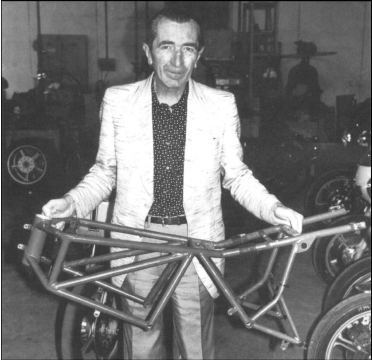
Legendary designer Taglioni showing off a triangulated Ducati frame. Current versions of such triangulated frames made in steel tubing have proved very successful in SuperBike racing against the generally more fashionable aluminium twin spar machinery. Such frames have a high structural efficiency. This particular frame is structurally incomplete without the engine. (Cathcart)
