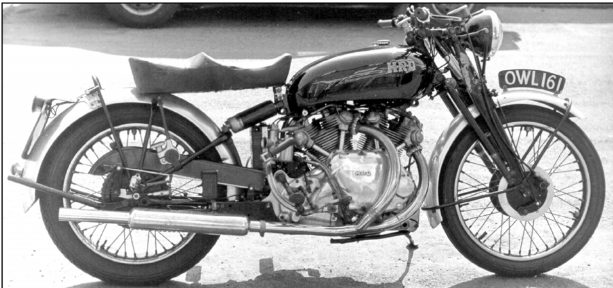
A series C Vincent-HRD Rapide with hydraulically damped Girraulic front fork and twin rear shock absorbers.
