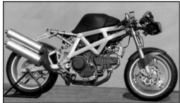
Both the V-twin engined Suzuki TL1000s (left) and the Bimota DB4 have frames with a beam down each side of the engine and as such have similarities to the normal twin-spar. The principal difference being that the spars are formed as triangulated structures rather than box sections.
