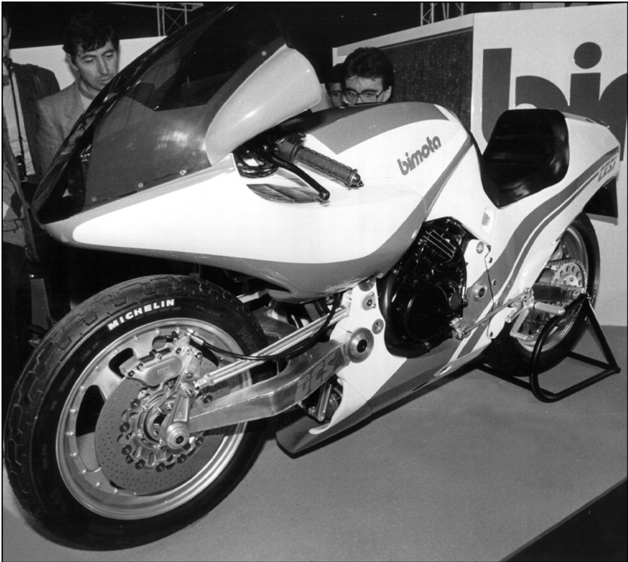
A 1983 Milan Show special – the student designed Bimota Tesi, with hydraulically operated steering. Geometrically similar to the Difazio, this design loaded the wheel spindle heavily in torsion when braking.
