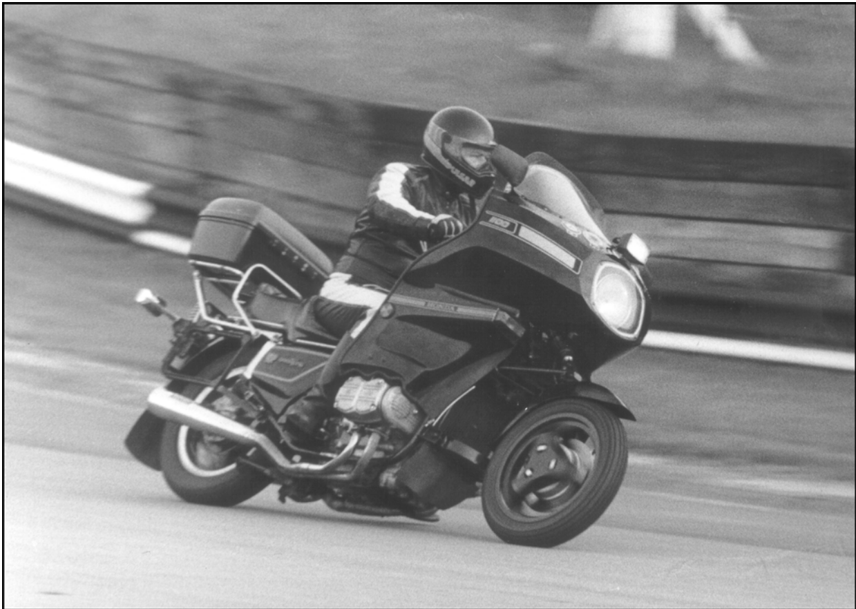
This is the Honda Gold Wing mentioned in the above text. Note the small 16" wheel at the front. For a number of reasons this machine had improved stability in gusting wind conditions. (photo: Kerry Dunlop)
