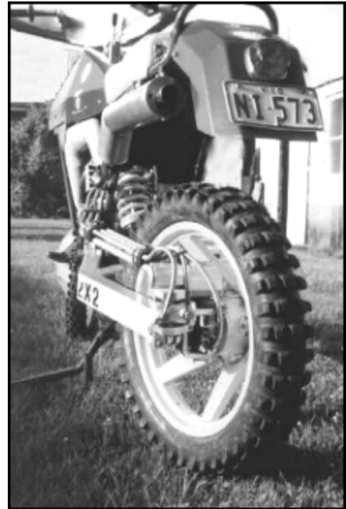
The Drysdale 2WS and 2WD motorcycle. The five piston radial hydraulic motor can be clearly seen in the hub of the front wheel shown on the left. Note also the cross-wise cylinder, which is for steering. The photo to the right shows the rear wheel in a steered position. This machine now resides in the Donington Collection Museum. (Drysdale)
