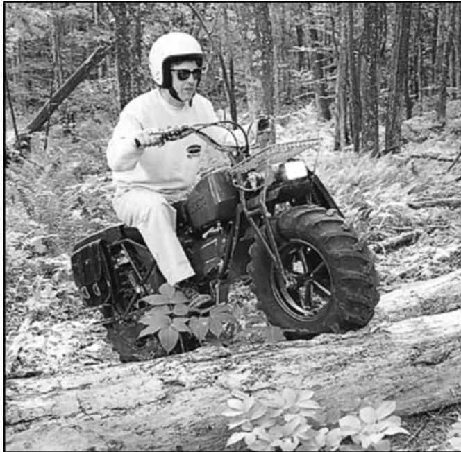
The 2WD Rokon makes riding over logs and through deep mud look easy. The model on the right has sealed aluminium disc wheels which with the balloon tyres allows the machine to be floated across deep streams. (Rokon)
