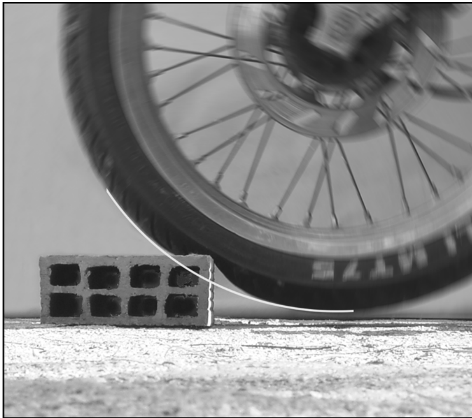
This photo shows a front wheel just after hitting a brick. The superimposed white line shows, what would have been, the undeformed shape of the tyre, demonstrating the bump absorbing properties of pneumatic tyres. The rim forces would have been destructive without this cushioning.
