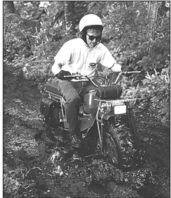
The 2WD Rokon makes riding over logs and through deep mud look easy. The model on the right has sealed aluminium disc wheels which with the balloon tyres allows the machine to be floated across deep streams. (Rokon)
