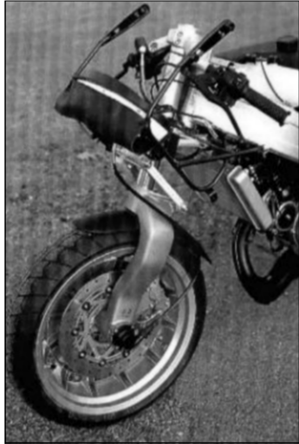
Gilera produced this system. Essentially this is a single leg telescopic suspension. Steering torque is transmitted via a folding linkage. This whole design is very much like that used on large aircraft landing gear.
