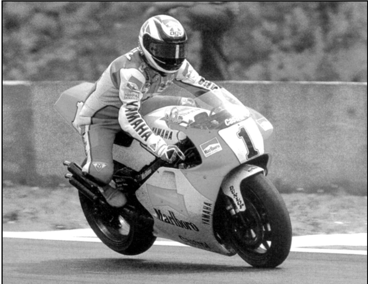
A perfect demonstration of both dive and load transference off the rear wheel as this bike is set up for a turn. Refer to fig. 9.37. (SM30)
