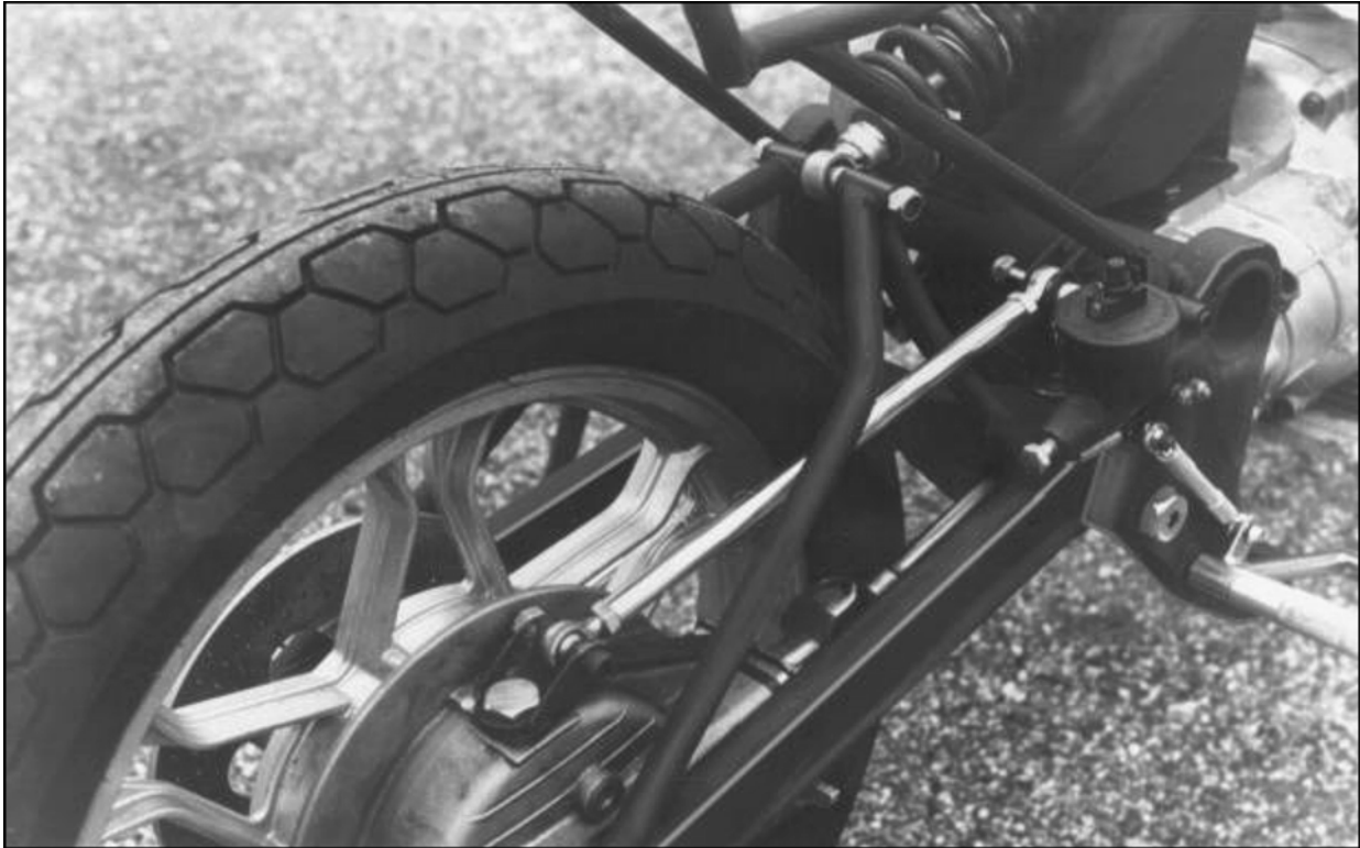
To prevent driving torque from extending the rear suspension excessively on this Foale-framed shaft-drive Guzzi the crown-wheel housing was made free floating and was connected to the main frame by a pivoted link above the swing-arm. Note the second Hooke's joint at rear of drive shaft. Guzzi themselves later adopted a similar solution, along with a very similar chassis, for their production sports machines, the V11 sport.
