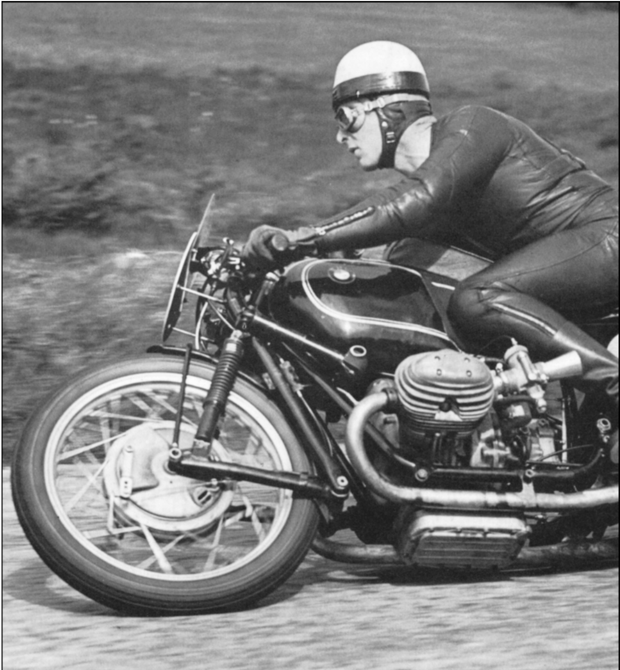
This 1956 Senior TT shot of Walter Zeller shows the Earles-type leading link front fork on the racing BMW (Renn-Sport). The brake-shoe back-plate was fixed to the left fork arm to provide a high degree of anti-dive. Note also the telescopic steering damper, unusual for the period. (MCW)
