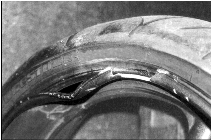
Fig 2.8. Not even the shock absorbing properties of the tyre are sufficient to prevent rim damage in all cases.
