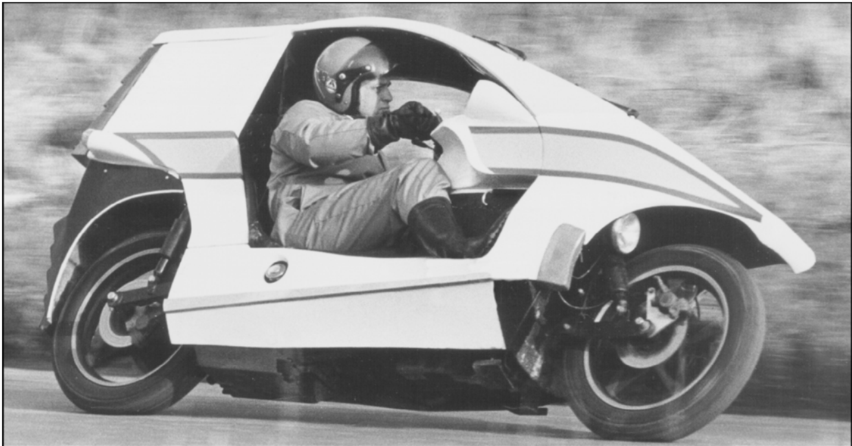
The Quasar in motion. Despite its weight and long wheel-base, 1800 mm., it had an agile cornering performance. Even with a relatively underpowered engine, the superior aerodynamics enabled a high top speed. Built to heavy construction standards, this machine has been shown to withstand frontal impacts better than conventional motorcycles. (Clive Dixon)
