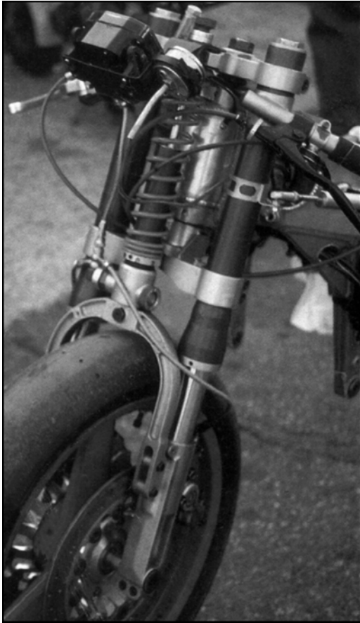
An unusual interpretation of the USD theme, made by Ceriani. Suspension is provided by a single spring and damper unit connected to a bridge piece connecting both legs together.
