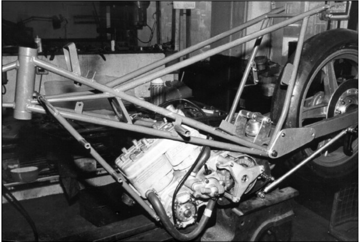
This Foale frame for a 250 cc Rotax-powered racer is of a simple triangulated type, as shown in fig. 10.4. The narrowness of the engine allowed this frame design, which is normally hard to implement with other engines.
